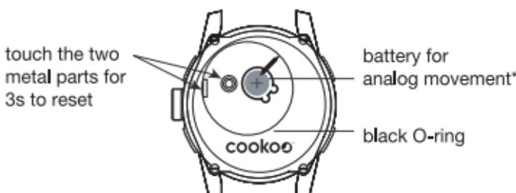
3. Insert the new battery and replace the battery cover (make sure the black O-ring is correctly positioned to ensure water resistance).
